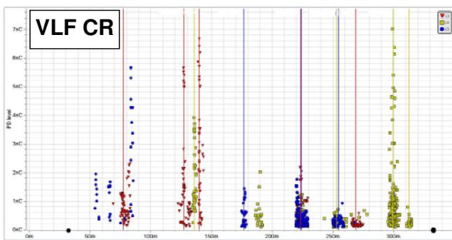
Figure 12. PD mapping of three cable phases done with VLF CR voltage  $\leq 10\text{kV}$  peak.
