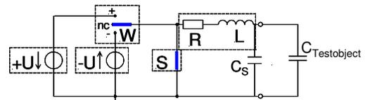
Figure 1. Principle of combined VLF CR & DAC at resonance phase.
