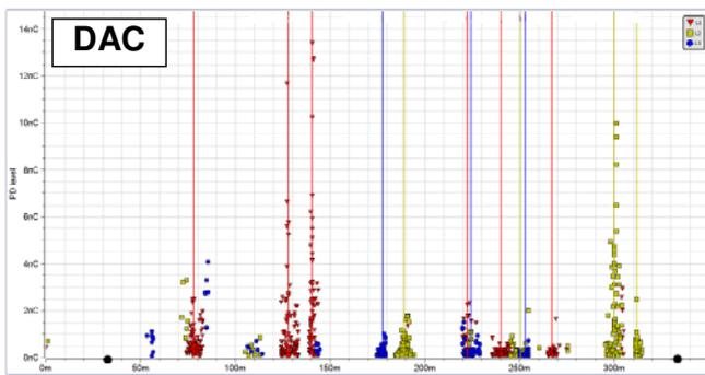
Figure 11. PD mapping of three cable phases done with DAC voltage  $\leq 10\text{kV}$  peak.
