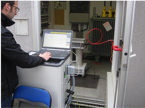
Figure 6. Test setup combined VLF CR and DAC voltage source and PD measurement device.
