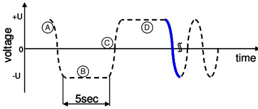
Figure 2. Timing diagram of VLF CR test cycle.
