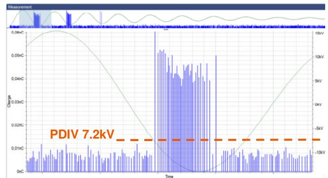
Figure 5. Corona defect at damped AC voltage.
