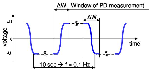
Figure 13. VLF cosine rectangular voltage distribution showing window of PD measurement.
