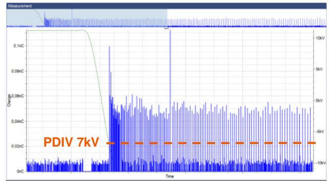
Figure 4. Corona defect at VLF cosine rectangular wave shape.
