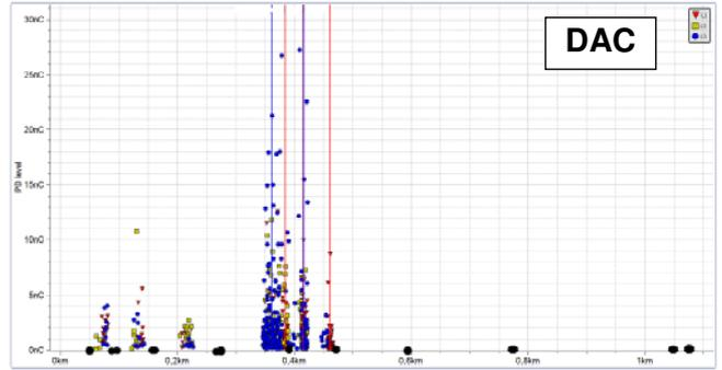
Figure 8. PD mapping of three cable phases done with DAC voltage  $\leq$  10kV peak.
