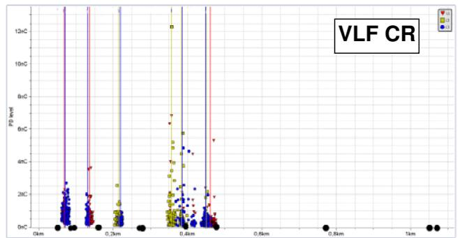
Figure 9. PD mapping of three cable phases done with VLF CR voltage  $\leq$  10kV peak.
